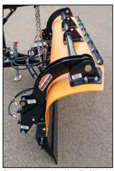
Flexing Arm: adjusts moldboard from 17" to 35" in height
