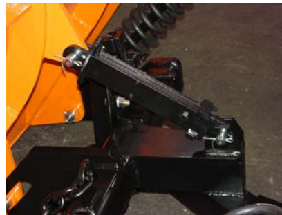
Adjustable pitch radius arm
