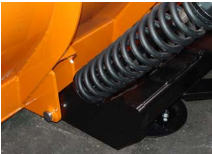
Spring and slotted trip assembly fully attached to push frame
