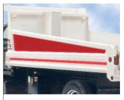
Almost double capacity with these sloping side boards. They are constructed of one-piece 12-gauge steel with 10-gauge top rail to take a real beating without yielding. Though they're tough, they are easy to install into builtin board pockets.
