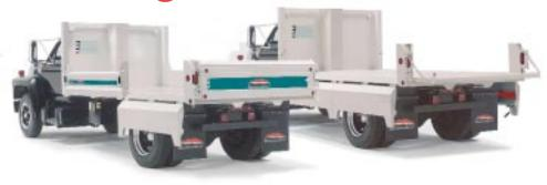
OPTIONAL: Split drop-sides add versatility of cargo handling from all sides. The complete side drops down or just the forward or aft sections on either side. A positive-latching system bonds the sections together for strength and rigidity when hauling dirt, gravel, sand and rubble. Sloped edges on the floor and side panels make them self-cleaning for easy closing.
