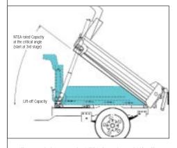
Illustrated above are the NTEA Capacity and Lift-off Capacity points of measure for the hoist data shown in the chart above.
