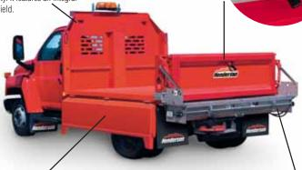
OPTIONAL quick-release, fold-down sides add convenience. The sturdy hinge is positioned beneath the body, out of the way of falling debris. Sloped surfaces on the sides and floor help shed debris during dumping.
