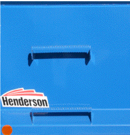
STEPS, GRAB HANDLE Weld-on access into the dump body. Universal brackets mount to body or around bracing.
