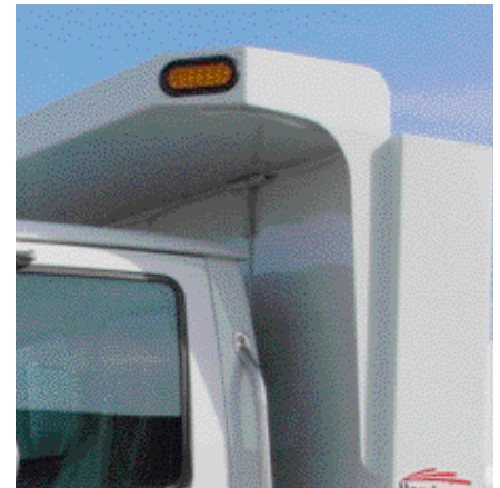
MARKER LIGHTS Two or four lights in numerous configurations. Shown with a 45-degree light in each corner.
