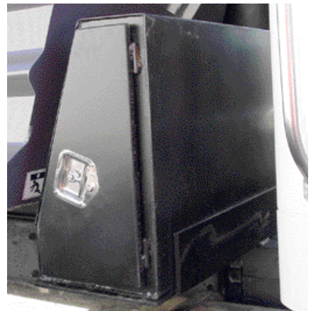
TRAPEZOIDAL TOOL BOX Tucks into space at front of sloped headsheet. 32" deep x 25" high.
