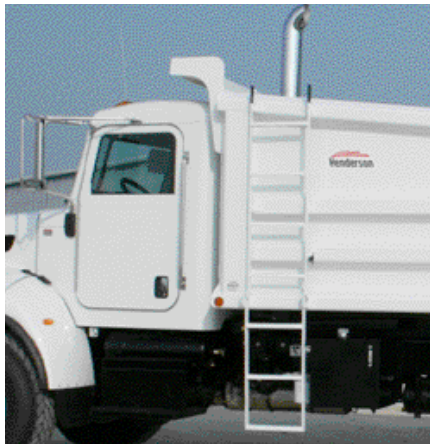
FOLD-UP LADDER Bottom half folds up and self locks. Rubber end covers for safe dump body entry.
