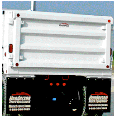
HORIZONTAL TAILGATE BRACING Two, three, or four additional horizontal tailgate-strengthening braces depending on tailgate height.
