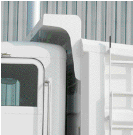
CABSHIELD Available 78" or 86" widths and 16", 22", 30" or 40" overhang.
