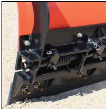
Adjustable Trip-edge: (6) adjustable torsion springs.
