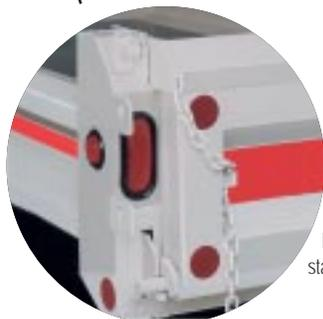
Full-depth rear corner posts are tied to 5" structural channel rear apron and have built-in stop/turn/tail lights. Built-in sideboard pockets are standard.
