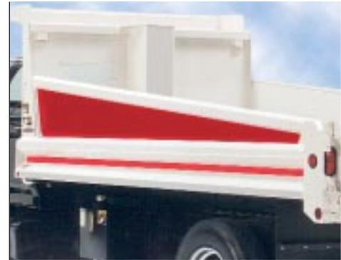
Almost double capacity with these sloping side boards. They are constructed of one-piece 12-gauge steel with 10-gauge top rail to take a real beating without yielding. Though they're tough, they are easy to install into built-in board pockets.
