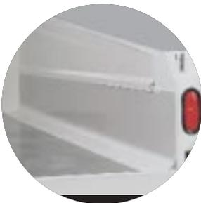
The unibody design features a one piece 3/16" high-tensile strength floor continuous seam welded to 12-gauge sides. A 2" floor-to-side radius eliminates load hang-up. (Optional sideboards shown)
