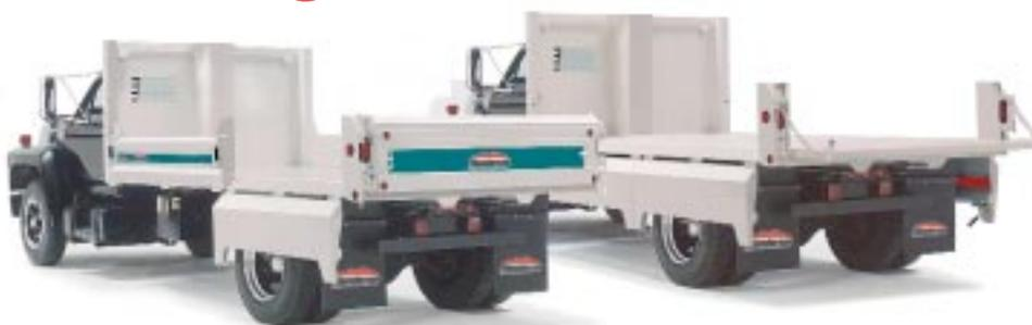
OPTIONAL: Split drop-sides add versatility of cargo handling from all sides. The complete side drops down or just the forward or aft sections on either side. A positive-latching system bonds the sections together for strength and rigidity when hauling dirt, gravel, sand and rubble. Sloped edges on the floor and side panels make them self-cleaning for easy closing.
